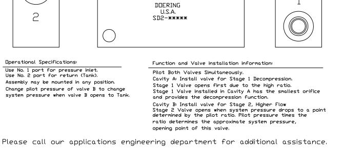
The SD2-\*\*\*\* is the part number for housing only. In addition, specify the valves.
