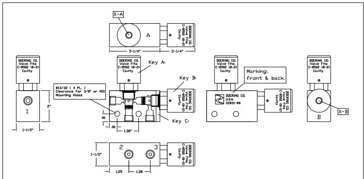
Key A: Illustrates Valve in housing cavity A, Doering Cavity C-8502 (8-2). Key B: Illustrates Valve in housing cavity B, Doering Cavity C-8502 (8-2). If another manufacturers cavity drawing or tooling is used, verify dimensions based on the Doering Company C-8502 (8-2) Cavity specifications, 1200630. Key C: S2831-## Housing
