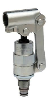
The seat is made from hardened steel for long operating life. Doering's standard plating, used on the DCHP102, has superior corrosion resistance. The piston is treated and hardened for improved wear and corrosion, heat and friction resistance.
