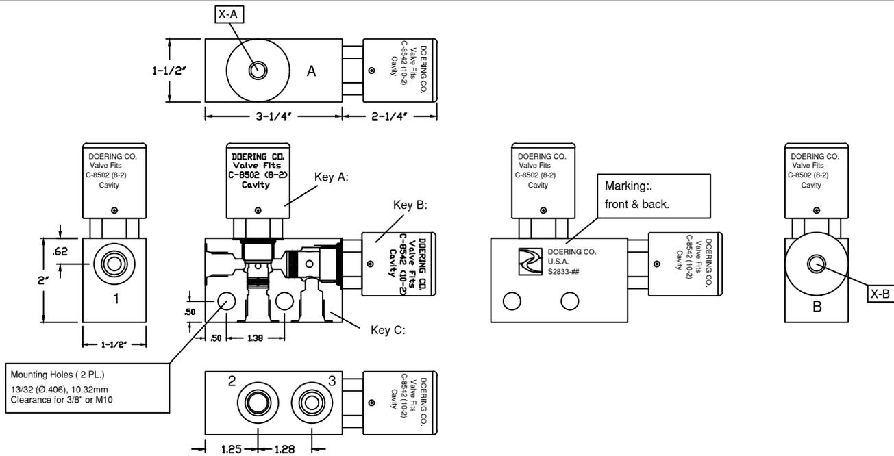
Key A: Illustrates Valve in housing cavity A, Doering Cavity C-8502 (8-2).
